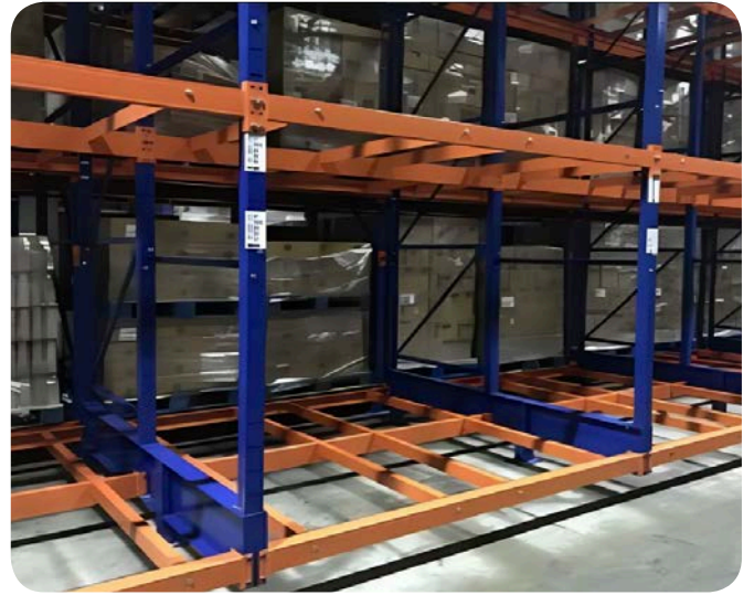
Double Deep Structural System
